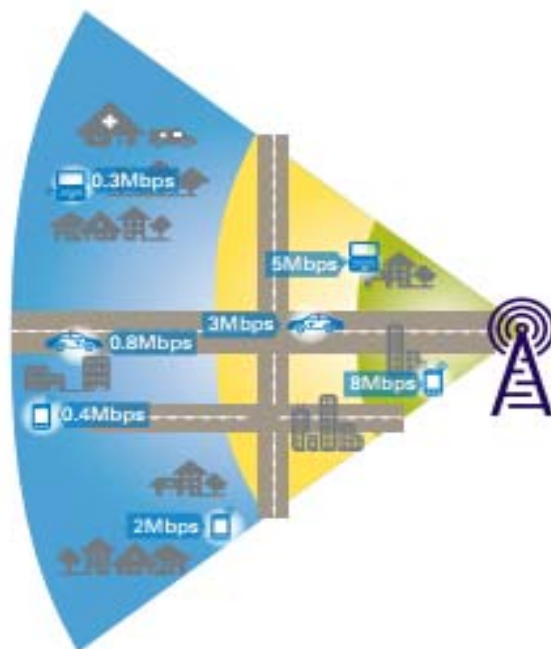
Figure 4-2: Snapshot of Instantaneous User Throughput within a Typical 10MHz Sector 53
